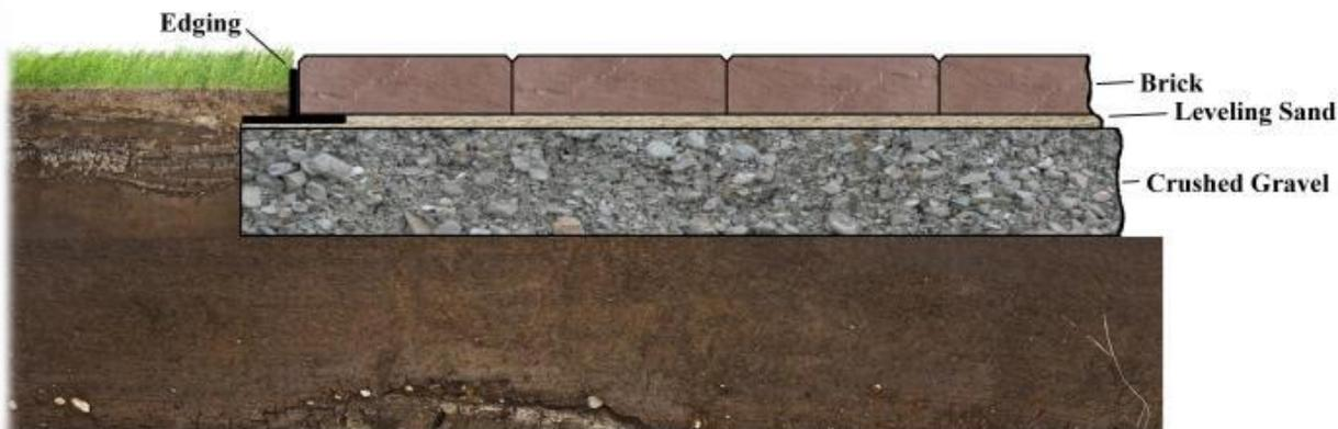
*A cross-section of a typical brick installation*
